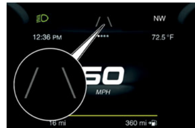
Lane Markings Not Detected
