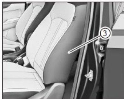
Front side airbag 3 is located outside the back of the front seat.
