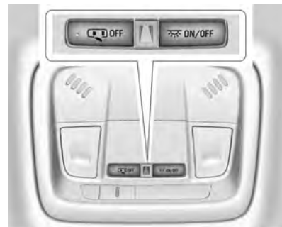
Dome Lamp Controls
