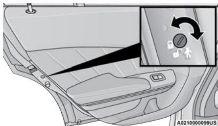
Child-Protection Door Lock Function
