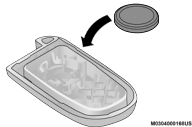
Key Fob Battery Replacement
