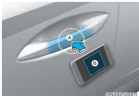
Ⓐ: Door handle authentication pad, Ⓑ: NFC Antenna
