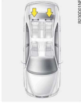
Securing a child restraint seat with child seat lower anchor system
