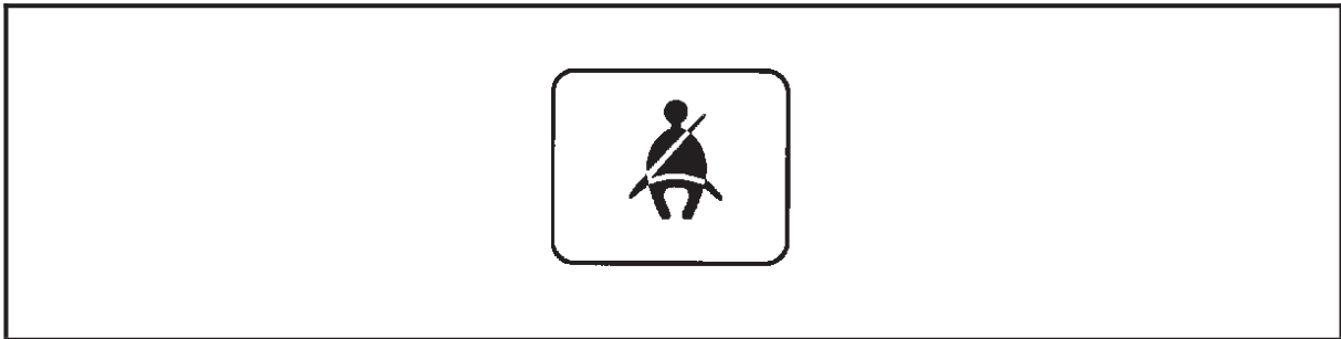
Safety belt warning light
