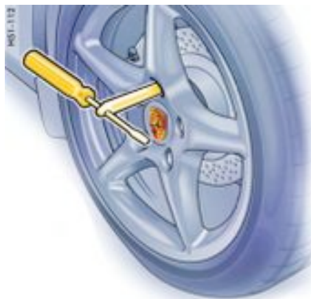
Screw in assembly aid for vehicles without Porsche Ceramic Composite Brake
