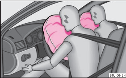
Fig. 119 Airbags rellenos de gas
