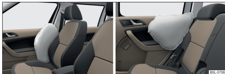
Fig. 13 Airbags rellenos de gas
