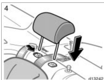
4. Outside anchor brackets only— Replace the head restraint.
