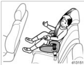
(C) BOOSTER SEAT INSTALLATION A booster seat must be used in forward-facing position only.
