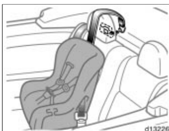
Follow the procedure below for a child restraint system that requires the use of a top strap.
