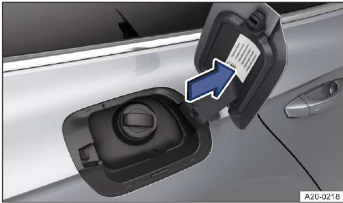
Fig. 1 On the inside of the tank flap: fuel information label (illustration).
