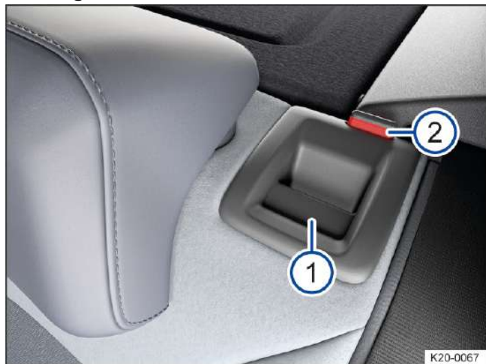
Fig. 1 In the rear seat backrest: release button.
