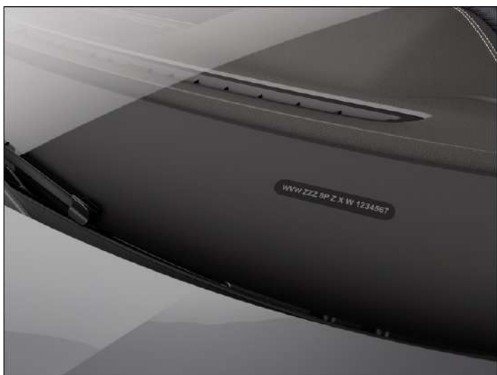
Fig. 1 In the windscreen: vehicle identification number.
