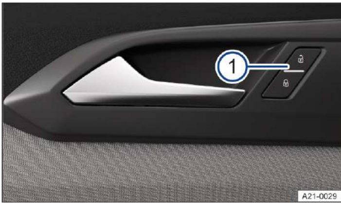
Fig. 1 In the driver door: central locking button (illustration).
