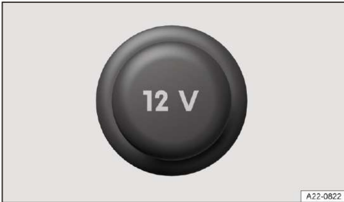
Fig. 1 In the front section of the centre console: 12-volt socket with removable cover (illustration).
