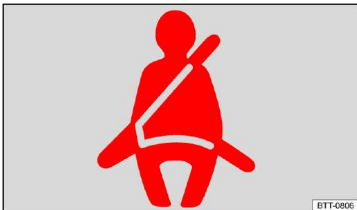
Fig. 1 On the instrument cluster display: warning lamp of the seat belt warning system.
