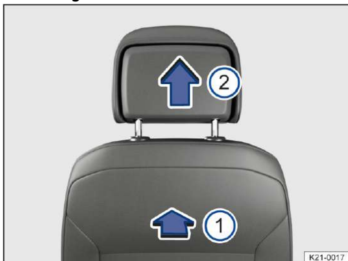
Fig. 1 Removing a front head restraint (illustration).
