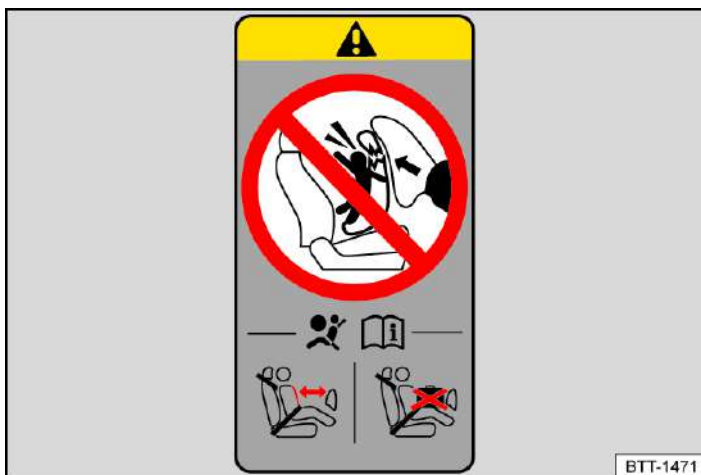
Fig. 2 On the B-pillar: airbag label(illustration).
