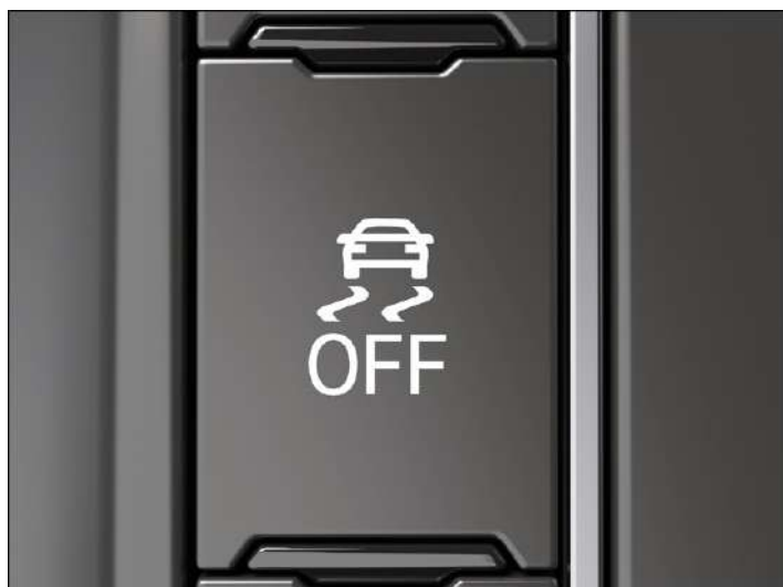
Fig. 1 In the centre console: button for switching ESC Sport on and off manually (depending on equipment).
