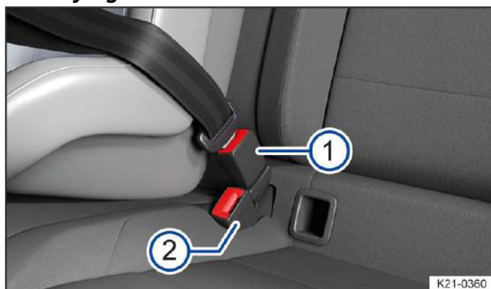
Fig. 1 In the second row of seats: position of the belt buckles (illustration).
