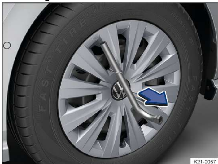
Fig. 1 Removing the wheel cover.
