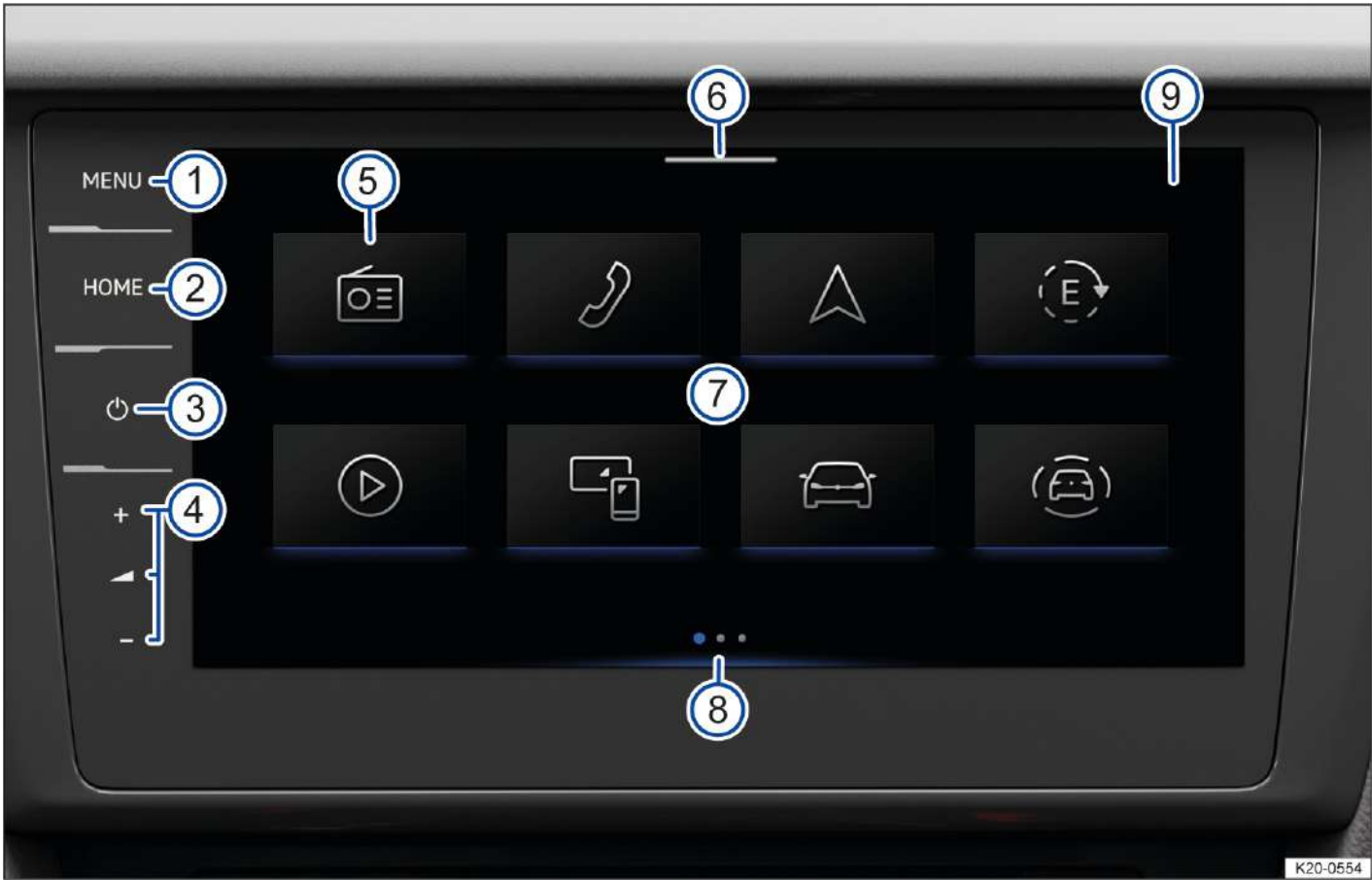
Fig. 1 Overview of the 9.2" Infotainment system.
