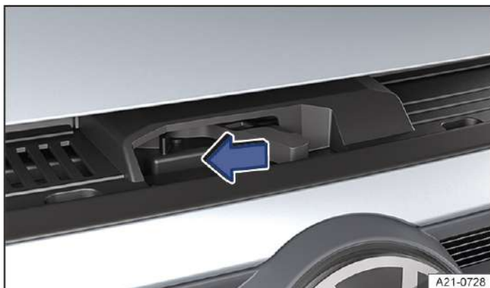
Fig. 2 Above the radiator grille: bonnet control lever.
