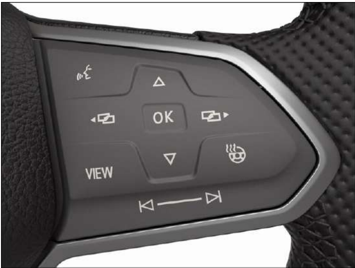
Fig. 2 Right side of the multifunction steering wheel: operating the digital instrument cluster Pro (variant 2).
