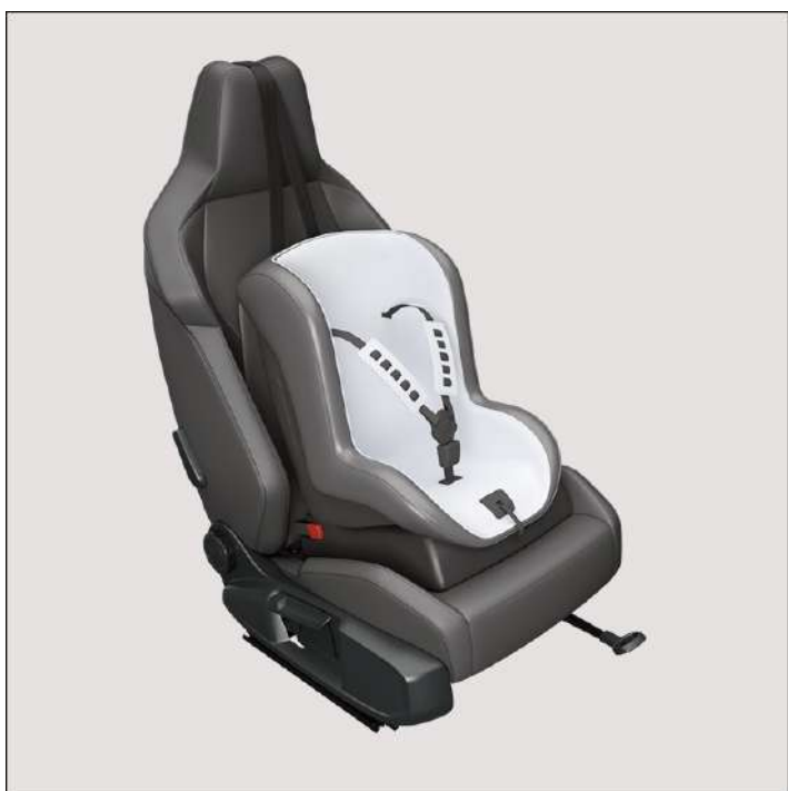
Fig. 3 In the backrest of the premium sport seat(without opening) on the front passenger side: routing for the top tether (illustration).
