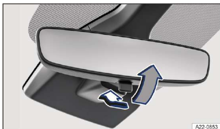
Fig. 2 On the windscreen: manual anti-dazzle interior mirror.
