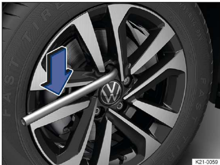
Fig. 1 Loosening wheel bolts.
