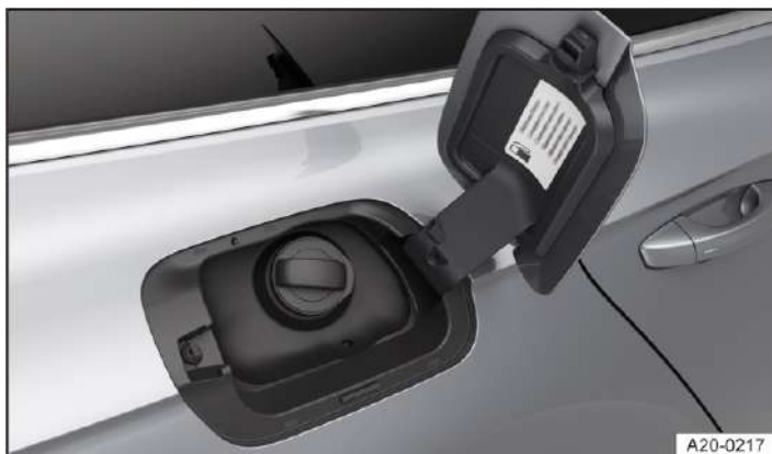
Fig. 1 Behind the tank flap: tank cap(illustration).
