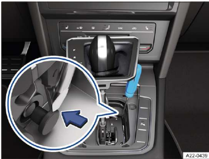
Fig. 1 In the centre console: releasing the selector lever lock manually (variant 1).
