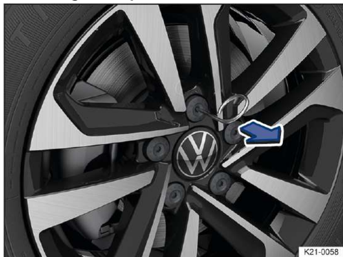
Fig. 1 Removing the wheel bolt caps.
