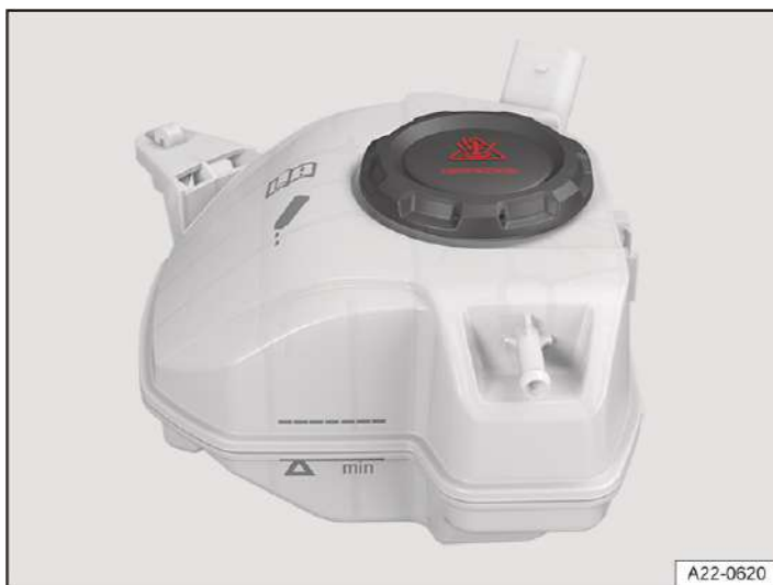
Fig. 2 In the engine compartment: markings on the coolant expansion tank (illustration).
