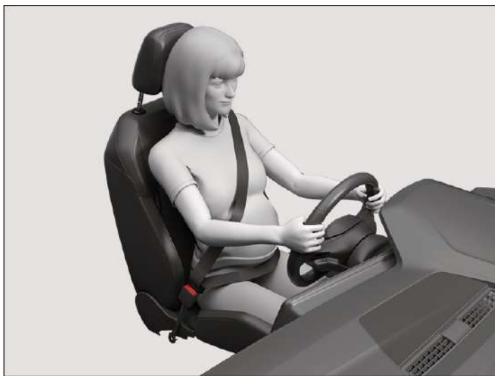
Fig. 2 Correct seat belt routing during pregnancy (illustration).
