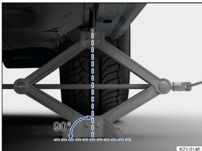
Fig. 2 Correct alignment of the jack.
