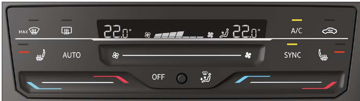
Fig. 1 In the upper part of the centre console: Climatronic air conditioning block(version 1).
