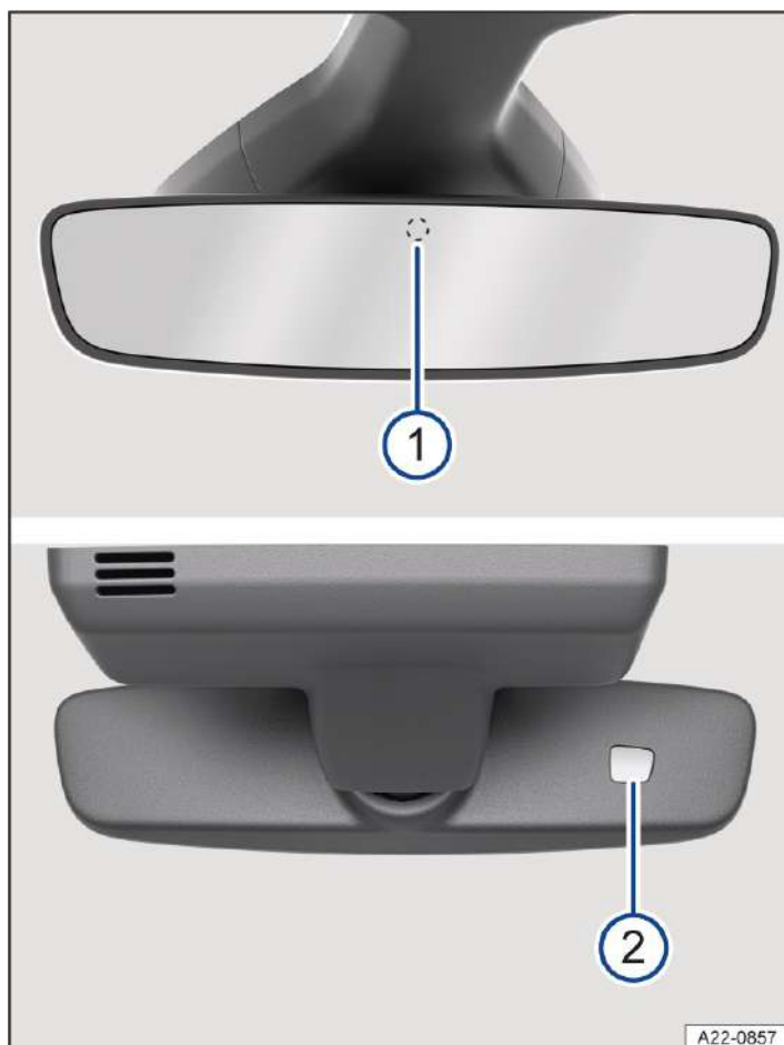
Fig. 1 On the windscreen: automatic anti-dazzle interior mirror.
