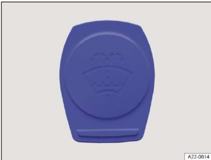
Fig. 1 In the engine compartment: washer fluid reservoir cap (illustration).
