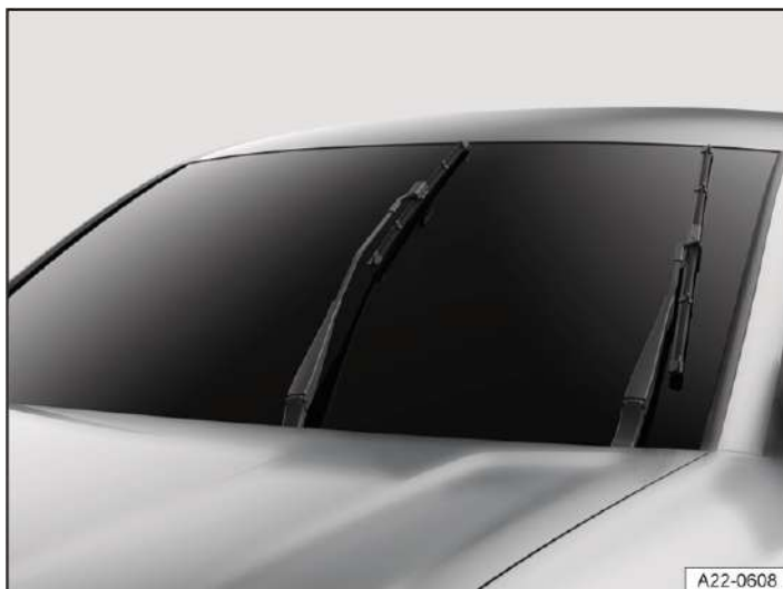
Fig. 1 Wipers in service position (illustration).
