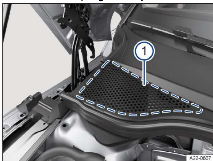
Fig. 1 Between the engine compartment and the windscreen: plenum chamber (illustration).
