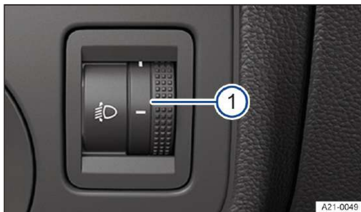
Fig. 1 Next to the steering wheel: control for headlight range control.
