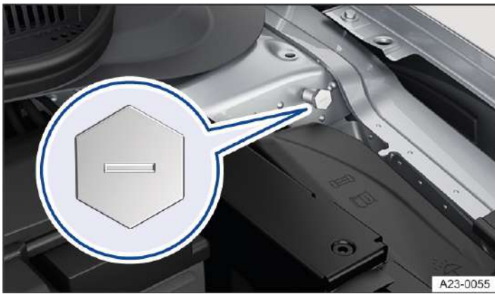
Fig. 1 In the engine compartment: jump-start connection point (earth).
