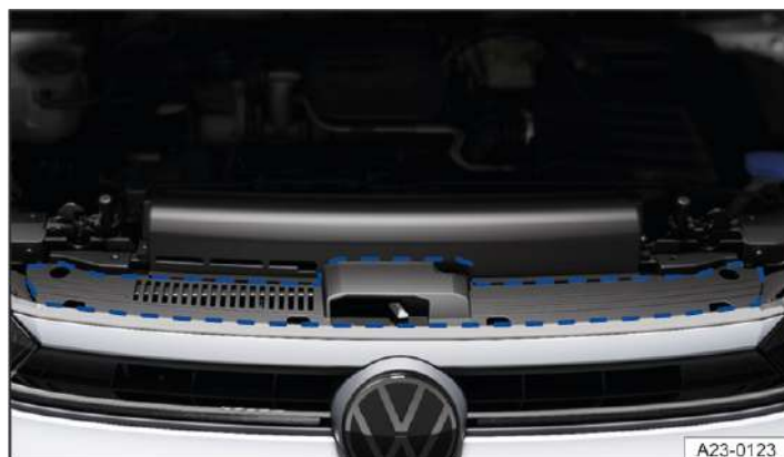
Fig. 1 In the marked area: location of the sticker for the engine oil standard and engine oil viscosity (illustration).
