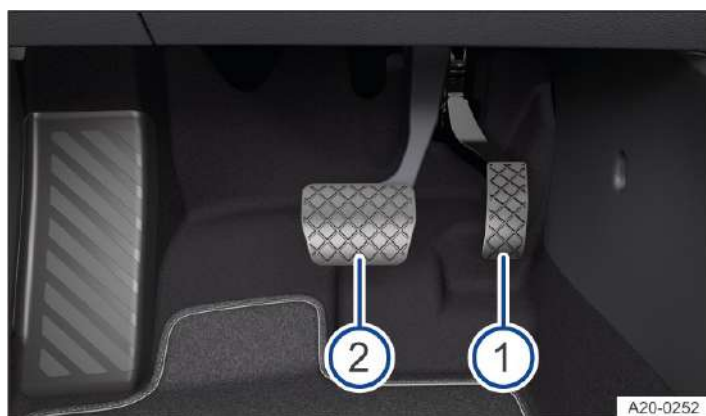
Fig. 2 In the footwell: pedals in vehicles with an automatic gearbox.
