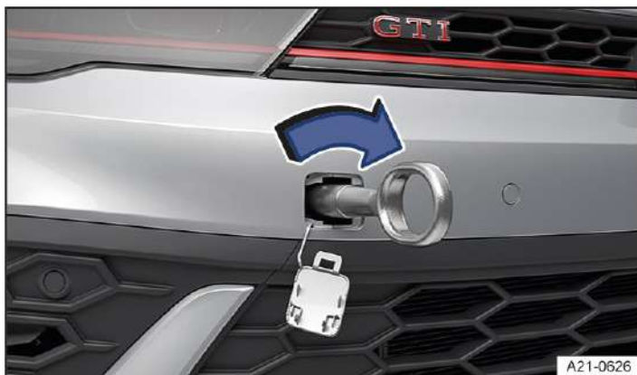
Fig. 4 In the front bumper on the right: screwing in the towing eye, variant 2.
