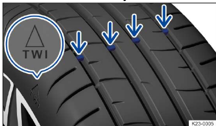
Fig. 1 In the tread grooves: tread wear indicator.
