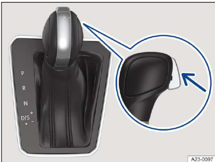
Fig. 1 In the centre console: selector lever of the dual clutch gearbox (illustration).
