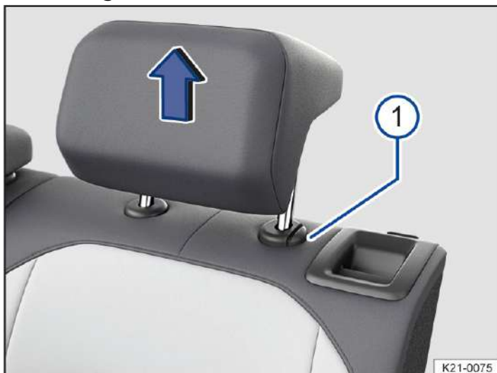
Fig. 2 Removing a rear head restraint (illustration).
