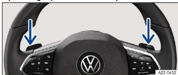
Fig. 2 Behind the steering wheel: paddles for Tiptronic.
